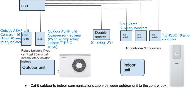
Cat 5 outdoor to indoor communications cable between outdoor unit to the control box (wpm controller) (From HSBC internal unit to external heat pump)
